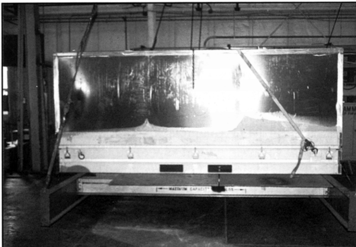
C-17 crash recovery airbag container pendulum impact test
