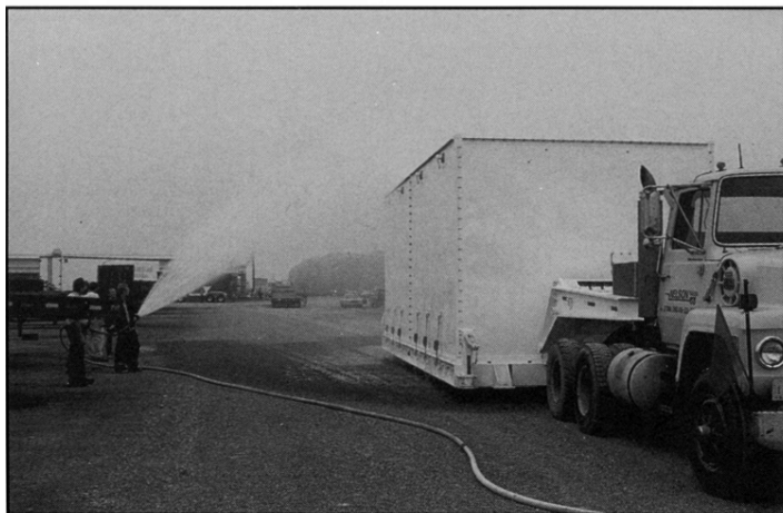
EOS AM-1 container cover rain test
