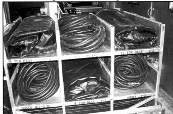
C-17 crash recovery airbag container cradle with hoses and airbags
