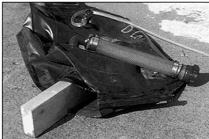
Failed Bag with 2 x 4 inserted in torn seam.
