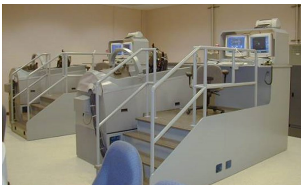
T-6A Unit Training Device (UTD) with Instructor Operation Station (IOS)
