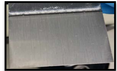
✓Increased surface area for bonding
