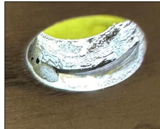
Horizontal Stab being Removed at AMARG (UP), Spar Chord Damage (LEFT)
