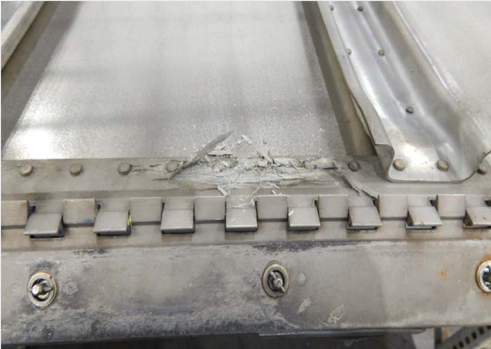
#2 Horse collar Hinge Corrosion
