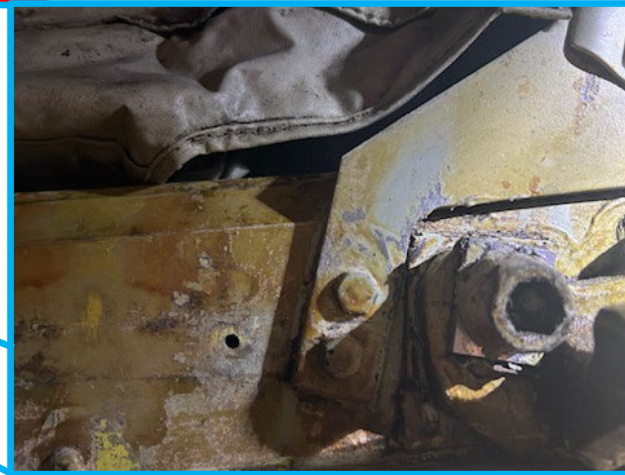
Flyswatter Bracket and Longeron Corrosion; found on post wash corrosion.
