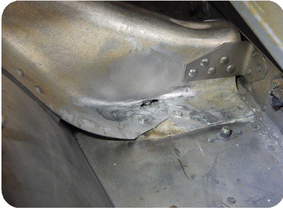
Engine Hat Channel Corrosion (Letter Check Find)
